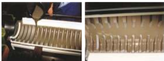
moulding of a hydrostatic tooth rack without machining
