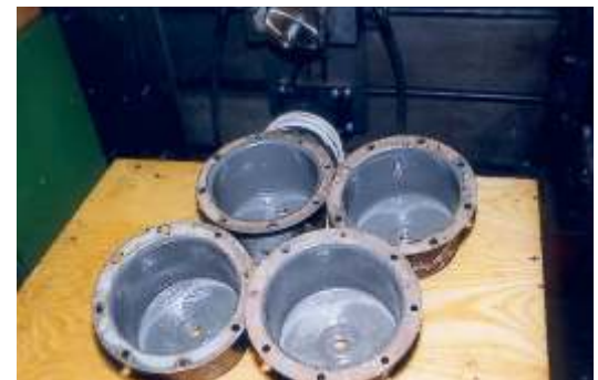
Interior coating of cover hoods with DIAMANT flexcoat FL grey
