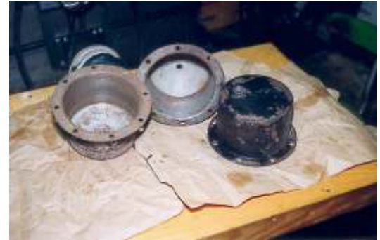
Interior coating of cover hoods with DIAMANT flexcoat FL grey
