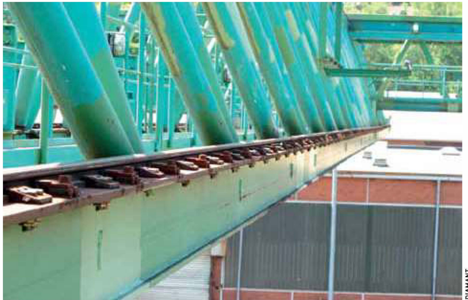
Outfield gantry crane before refurbishment: crane rail is wavy and tilted.
