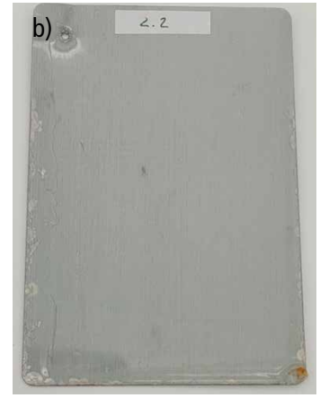
Fig. 6: Exposure tests in 5% NaCl solution at 25 °C after 4 weeks: Steel sheet with (a) severe and (b) minor corrosion damage
